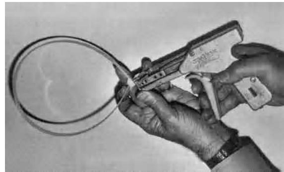
Figure B — Nonmetallic Duct Clamp
