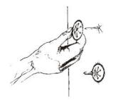
Insulation can be impaled immediately and firmly locked with locking washers, but maximum strength of adherence is achieved afetr 24 hours. If necessary, cover the pin with protective cap.
