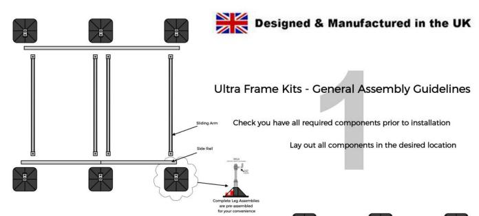
Guide the Sliding Arms onto the Side Rails, then fix at the desired position. For ease of installation we recommend installing the Sliding Arms with the open side up.
