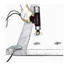
Press the pin through the insulation until the point meets the sheet metal and press the trigger
