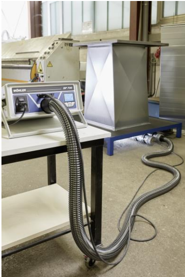
Fig. 12: Example: Measurement according to DIN EN 15727
