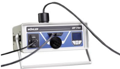
Fig. 13: Negative pressure measurement with flow rate <math>< 0.3 \text{ l/s}</math>
