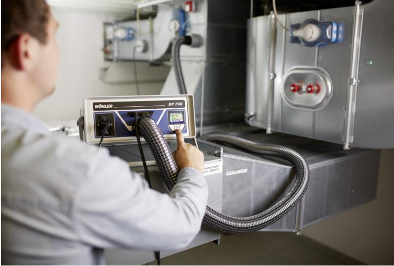
Fig. 11: Example: positive pressure measurement without adapter
